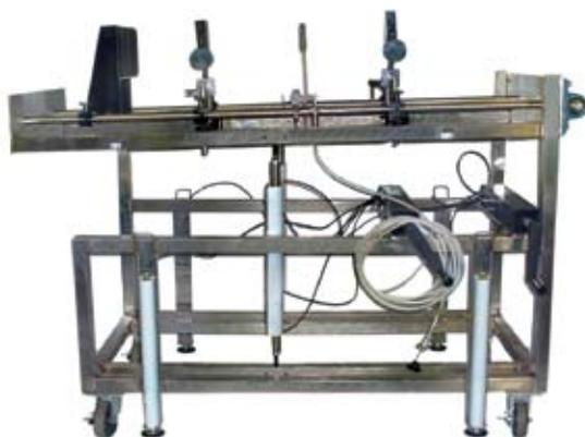
**Remote Firing Stand** shown with the protective cover removed for illustration purposes only.
